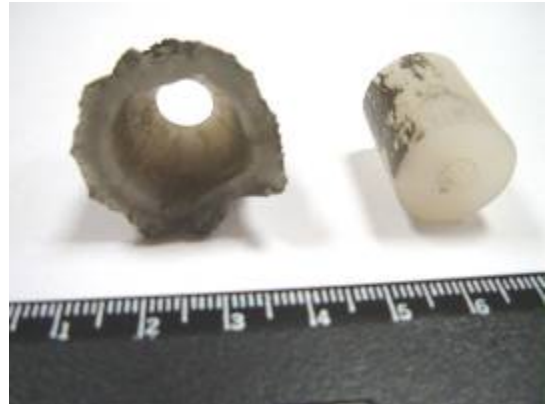
Explosive Inversion: Target samples are literally turned inside out from the explosion.
