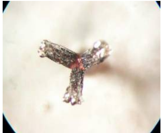
Explosion: A clean explosion of a target sample from internal plasma pressure.
